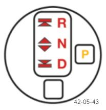
When the ignition is switched "ON" and the transmission control module *does not detect the P position*, position N will flash in addition to the Check Control message "emergency release may be operated". This can also occur if the Bus is awake, KL15 is ON and the Bus activation line is "high".
